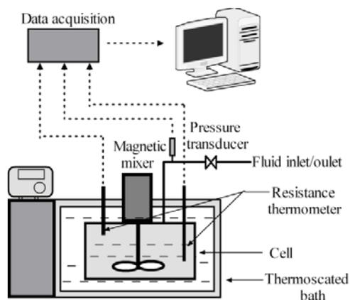
Fig. 1: Schematic of the experimental apparatus used for phase equilibrium measurements
