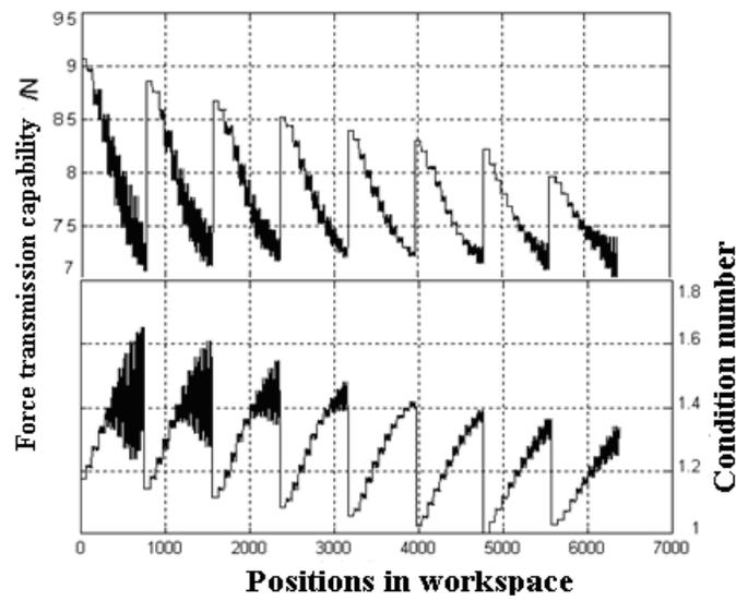
Fig. 6: Curve of force transmission capacity/condition number in workspace
