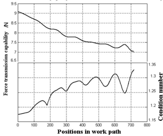
Fig. 5: Curve of force transmission capacity/condition number in work path
