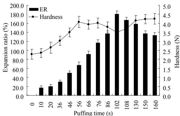
Fig. 5: Variation of hardness and expansion ratio for maitake mushroom samples during the PMVP process (initial moisture content:  $40 \pm 1.0\%$ ; microwave intensity: 150 W/g; vacuum pressure:  $-70 \pm 1.5$  kPa, pulse ratio 1.2)
