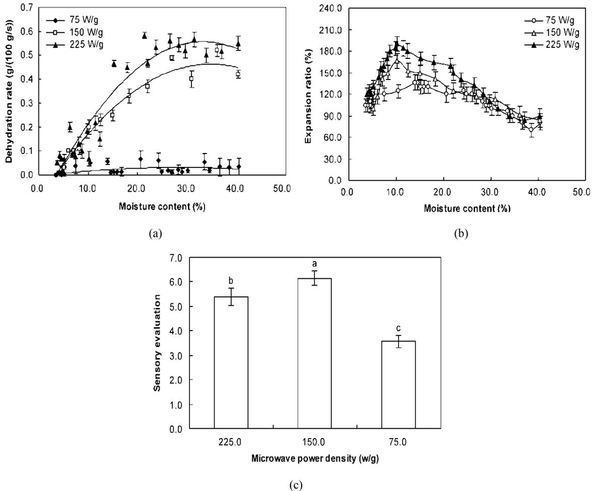
Fig. 2: Effect of microwave power intensity on puffing characteristics; (a): dehydration rate; (b): expansion ratio and; (c): sensory evaluation (initial moisture content:  $40\pm 1.0\%$ ; vacuum pressure:  $-60\pm 1.5$  kPa; pulse ratio 1.2. values bearing different lowercase letters (a-c) are significantly different (Duncan,  $p < 0.05$ ))
