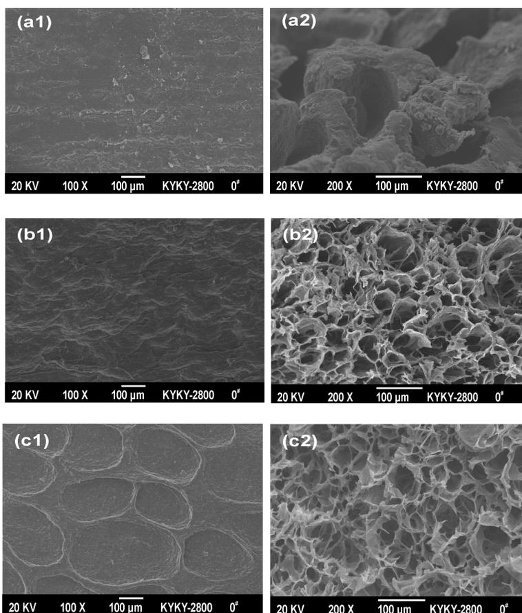
Fig. 6: Effect of the PMVP process on the microstructure of the maitake mushrooms. SEM images of the surface microstructures (a1), (b1) and (c1) expanded 100 times; SEM images of the cross-section microstructures (a2), (b2) and (c2) expanded 200 times; (a1) and (a2) are the microstructures after preliminary drying; (b1) and (b2) are the microstructures after puffing for 70 s; (c1) and (c2) are the microstructures after expanding to a moisture content of  $7 \pm 1.0\%$
