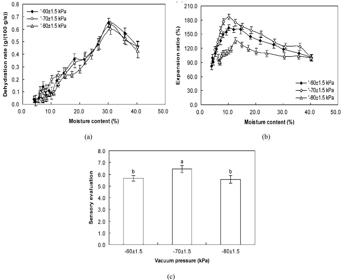
Fig. 4: Effect of vacuum pressure on puffing characteristics by initial moisture content; (a): dehydration rate; (b): expansion ratio and; (c): sensory evaluation (initial moisture content:  $40\pm 1.0\%$ ; microwave intensity: 150 W/g; pulse ratio 1.2. values bearing different lowercase letters (a–b) are significantly different (Duncan,  $p < 0.05$ ))
