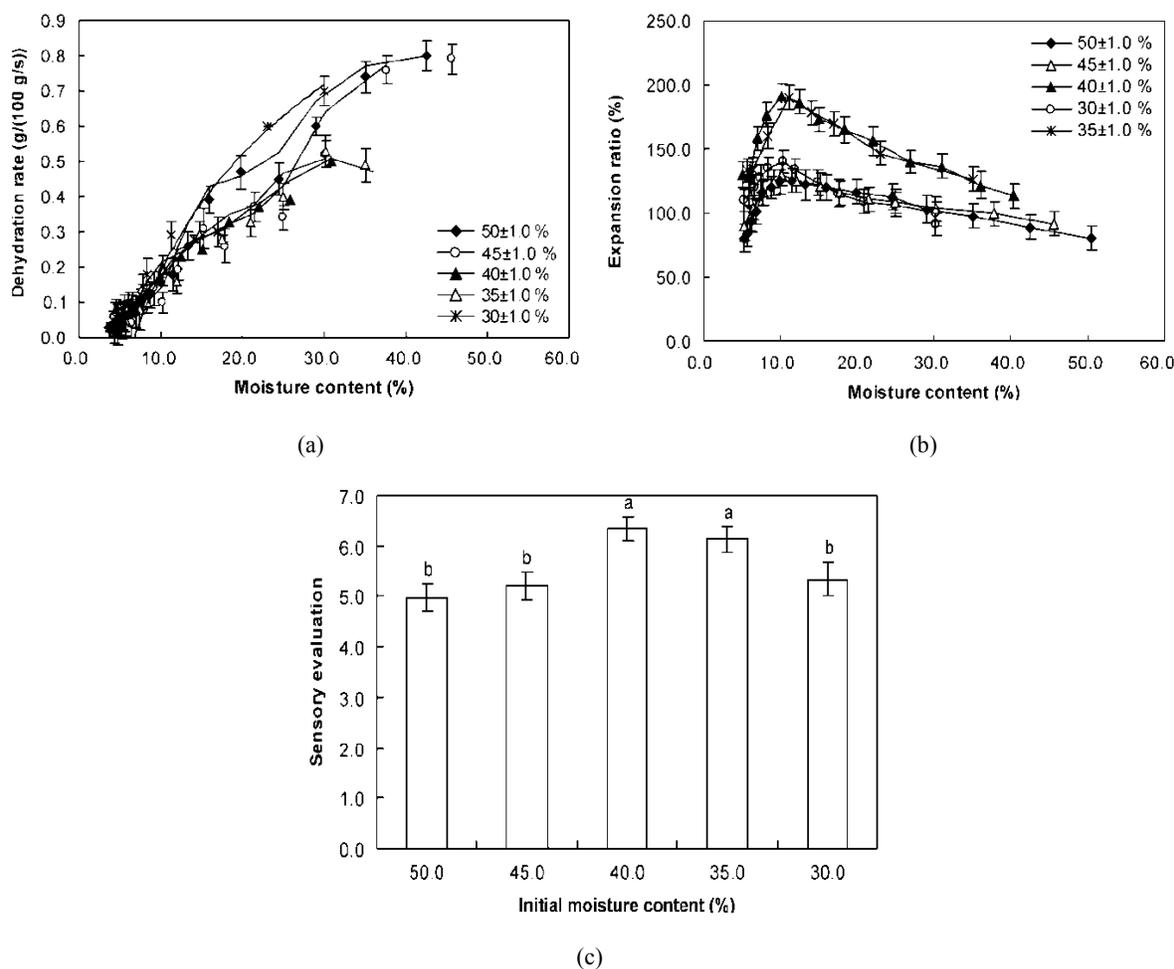
Fig. 3: Effect of initial moisture content on puffing characteristics by initial moisture content; (a): dehydration rate; (b): expansion ratio and; (c): sensory evaluation (microwave intensity: 150 W/g; vacuum pressure:  $-70\pm 1.5$  kPa; pulse ratio 1.2. values bearing different lowercase letters (a–b) are significantly different (Duncan,  $p < 0.05$ ))
