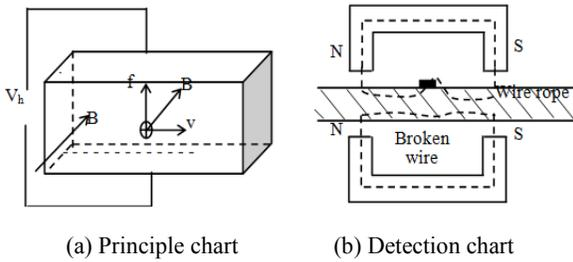
Fig. 1: NDT principle chart of broken wire rope
