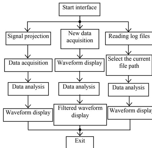
Fig. 3: The flow chart of software
