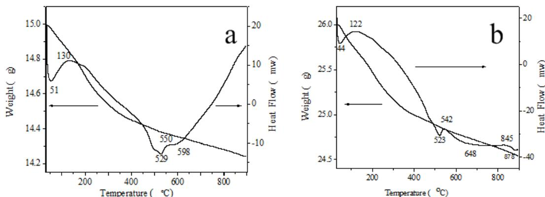
Fig. 1: TG-DSC curve of  $\text{CaMoO}_4$ ; (a): No addition PEG; (b): Addition PEG
