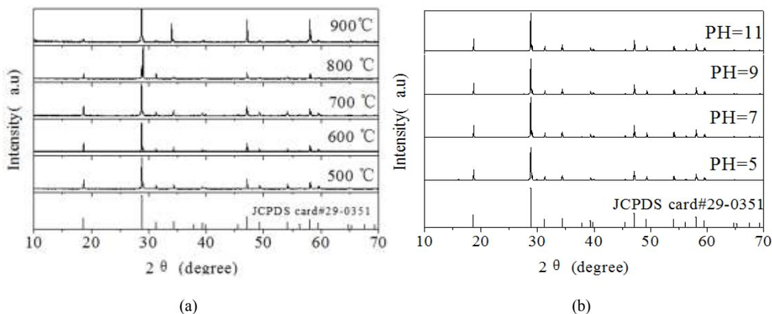
Fig. 2: XRD patterns of the  $\text{CaMoO}_4$  samples (addition PEG) obtained at; (a): Different firing temperature; (b): Different PH value
