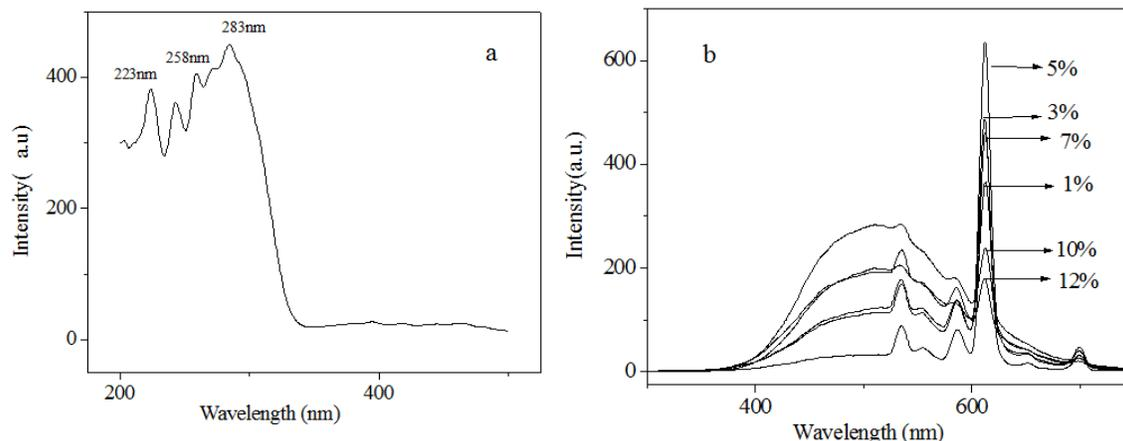
Fig. 3: Excitation spectrum of CaMoO<sub>4</sub>: Eu<sup>3+</sup> with different amount of Eu<sup>3+</sup> doping under 258 nm excitation
