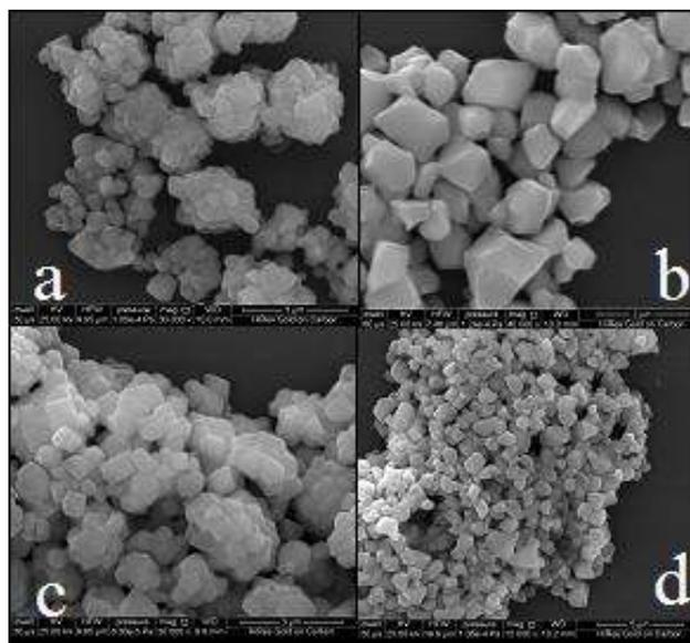
Fig. 4: SEM images of CaMoO<sub>4</sub>; (a, b): Fired at 500 and 700°C, respectively (no addition PEG); (c, d): CaMoO<sub>4</sub> and CaMoO<sub>4</sub>: Eu<sup>3+</sup> (5%) fired at 700°C (addition PEG)
