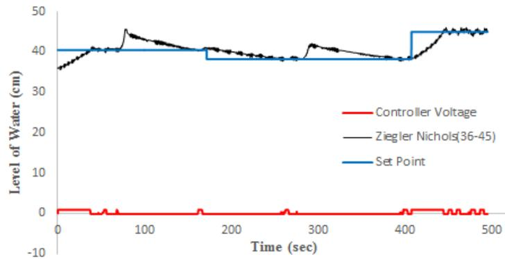
Fig. 5f: ZN tuned AMBGS controller's regulatory response for region 36-45cm
