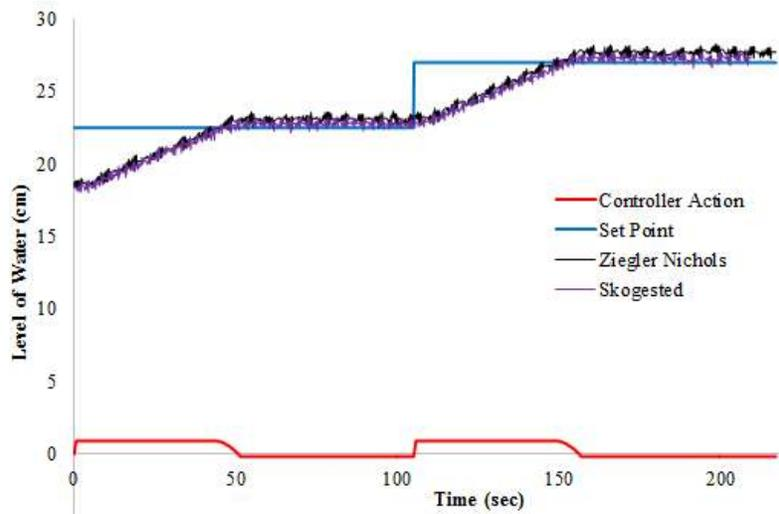
Fig. 6b: Servo response comparison of Skogestad's and ZN tuned AMBGS controllers for region 18-27cm
