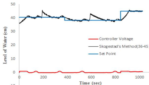
Fig. 5c: Skogestad's tuned AMBGS controller's regulatory response for region 36-45
