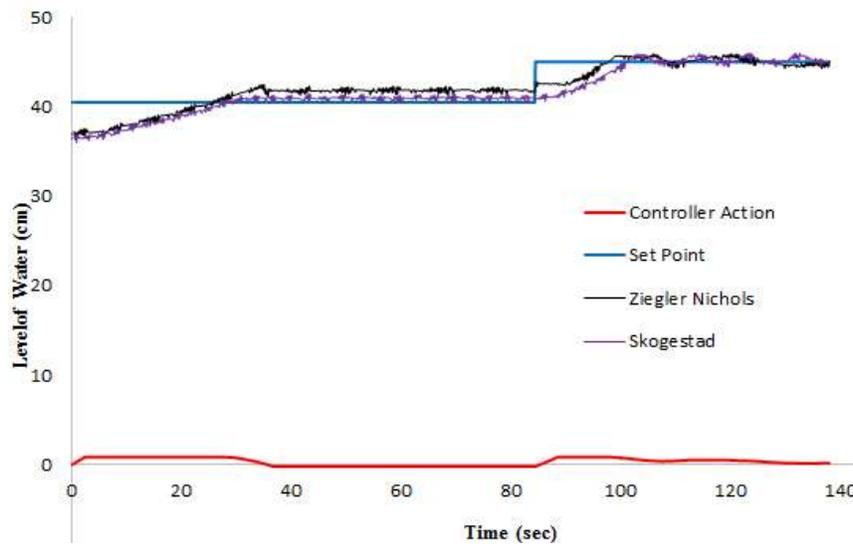
Fig. 6c: Servo response comparison of Skogestad's and ZN tuned AMBGS controllers for region 36-45cm
