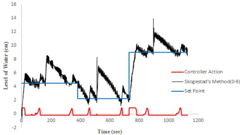
Fig. 5a: Skogestad's tuned AMBGS controller's regulatory response for region 0-9
