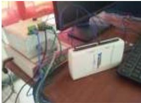
Fig. 3: Interfaced NI-DAQmx 6211 data acquisition module card
