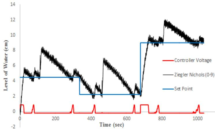
Fig. 5d: Ziegler Nichols tuned AMBGS controller's regulatory response for region 0-9
