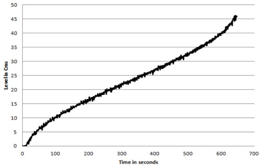
Fig. 1: S-shaped open loop input-output response curve
