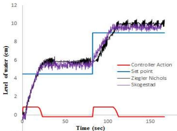
Fig. 6a: Servo response comparison of Skogestad's and ZN tuned AMBGS controllers for region 0-9cm
