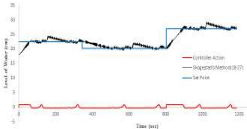
Fig. 5b: Skogestad's tuned AMBGS controller's regulatory response for region 18-27
