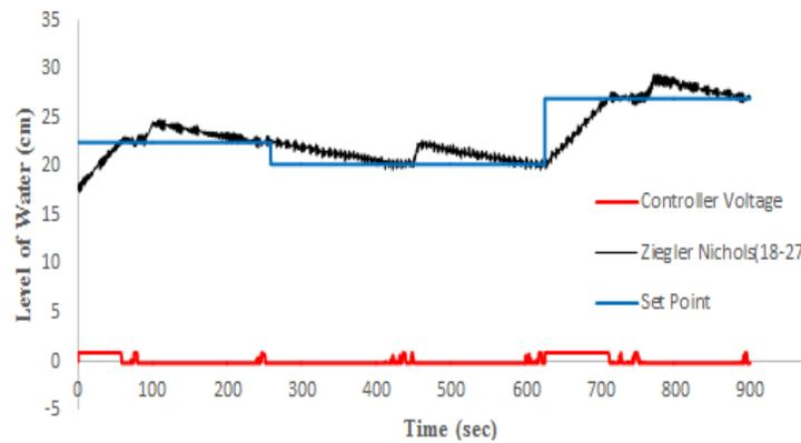
Fig. 5e: Ziegler Nichols tuned AMBGS controller's regulatory response for region 18-27cm
