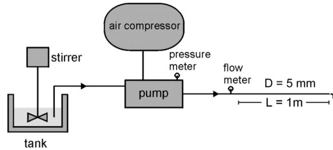
Fig. 1: Device for pumping grouts through capillary tube
