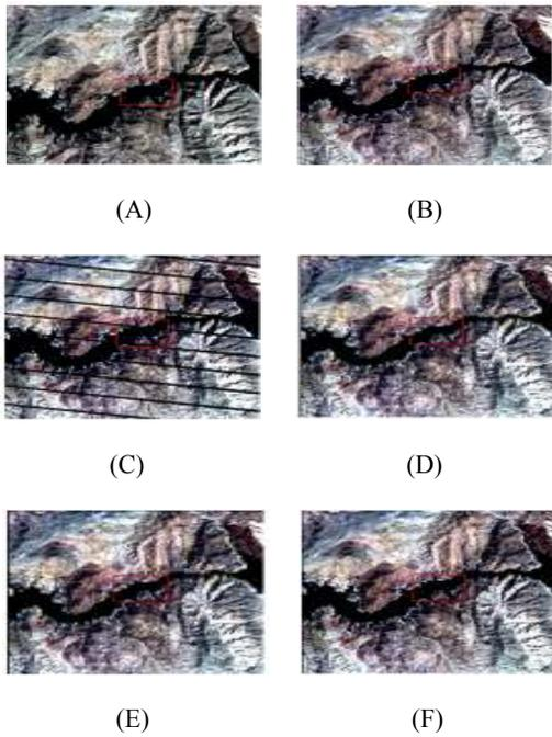
Fig. 2: Red-green-blue composites of Landsat 7 SLC-on image for the simulation captured in 2003; (A): Target image in May 26; (B): SLC-on fill image of March 9. Panel; (C): The simulated SLC-off based on image from A. PANELS; (D-F): The results of mean, IDW and LLHM approaches respectively
