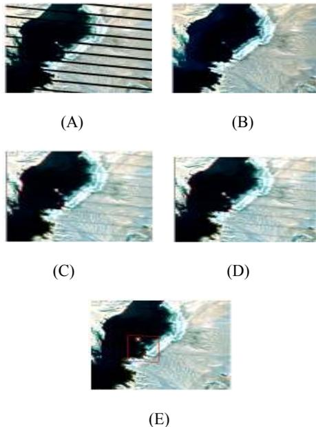
Fig. 4: Experiment results on actual Landsat 7 SLC-off image (taken in 2003); (A): The target image (September 17); (B): Fill image (April 26). The obtained result; (C): From mean method; (D): From IDW method; (E): From LLHM method
