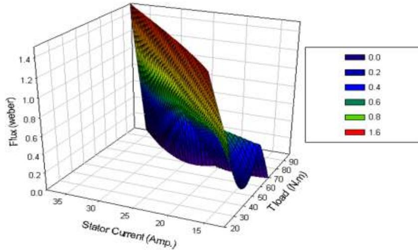
Fig. 14: The optimal flux vs. stator current for various loads
