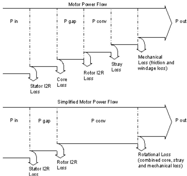
Fig. 2: Power flow in an induction motor
