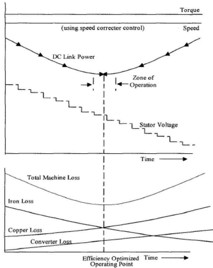
Fig. 1: Efficiency optimized operating point
