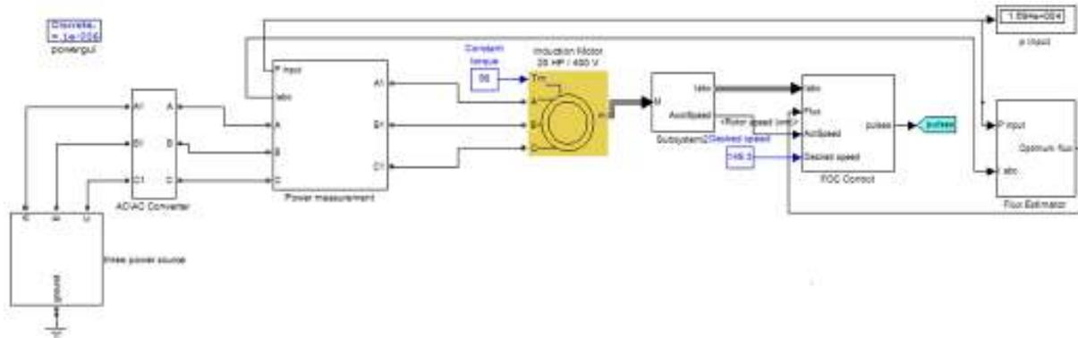
Fig. 5: MATLAB simulation model of optimal control
