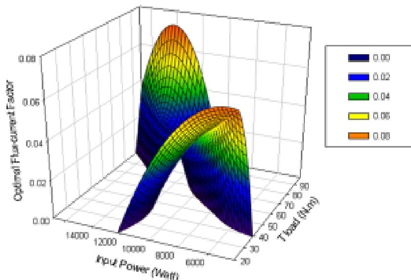
Fig. 13: The optimal flux-current vs. power input for various loads
