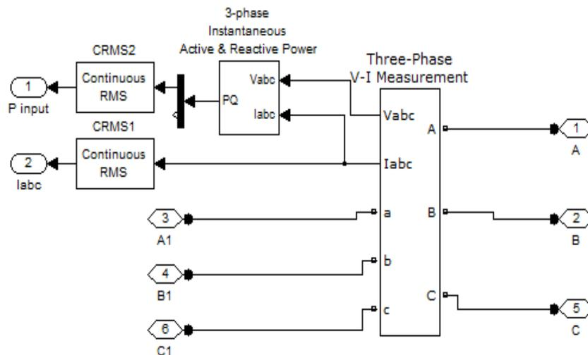
Fig. 8: Power measurement block
