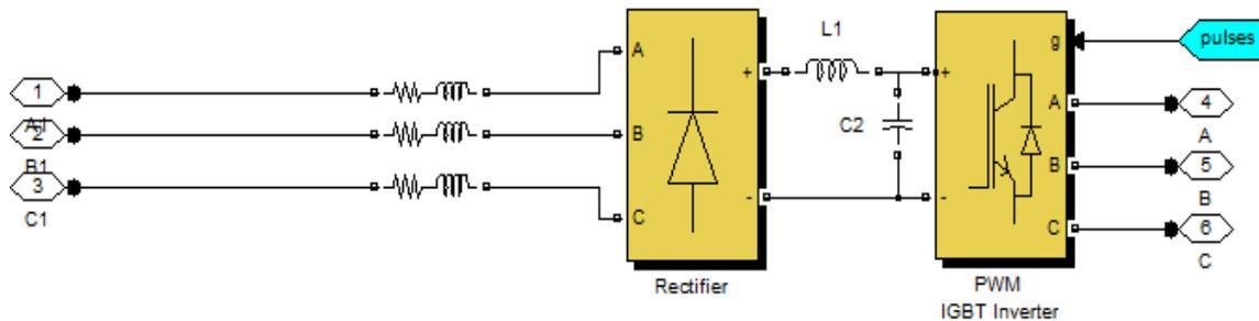
Fig. 7: AC to AC converter modelling
