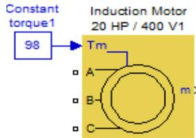
Fig. 9: Twenty hp induction motor modelling
