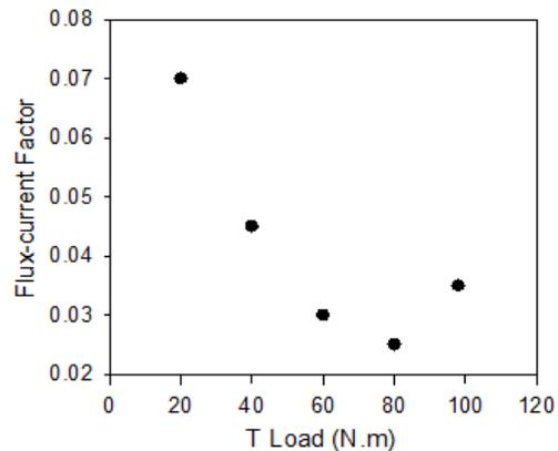
Fig. 12: Optimal flux-current factor versus load (N.m)
