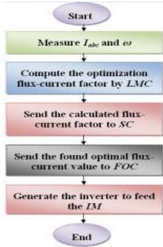
Fig. 3: The algorithm of presented optimization system
