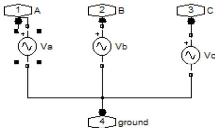
Fig. 6: Three phase power source modelling
