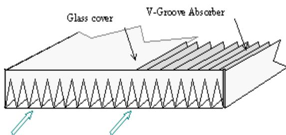
Fig. 15: Configuration of the V-groove absorber
