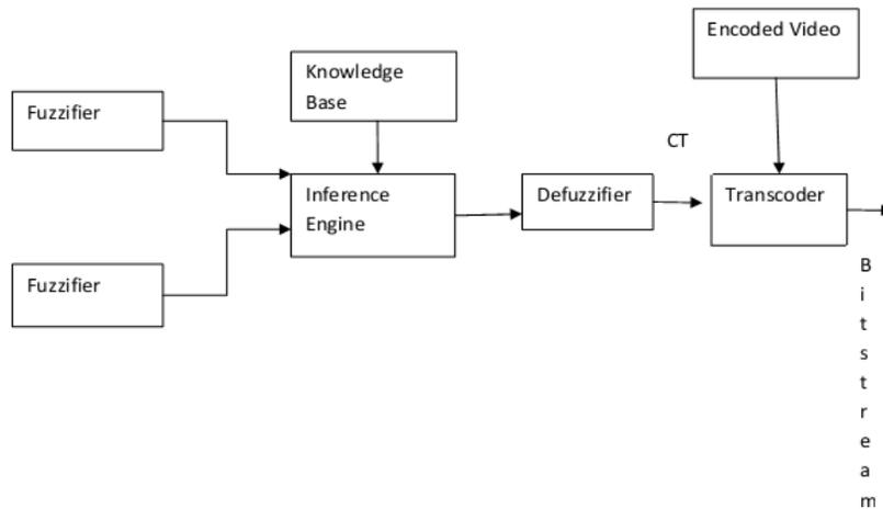
Fig. 3: Block diagram of fuzzy logic controller
