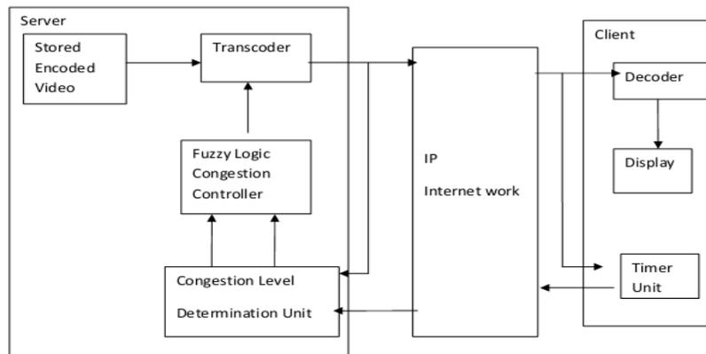
Fig. 7: Video streaming architecture
