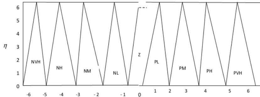
Fig. 6: Output membership function (W)
