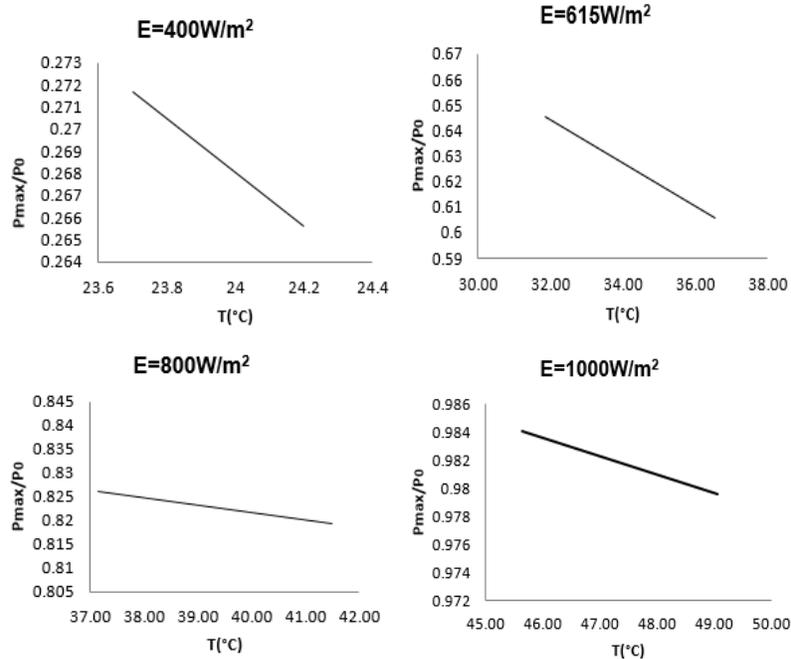
Fig. 14: Influence of temperature on the degradation at constant radiation
