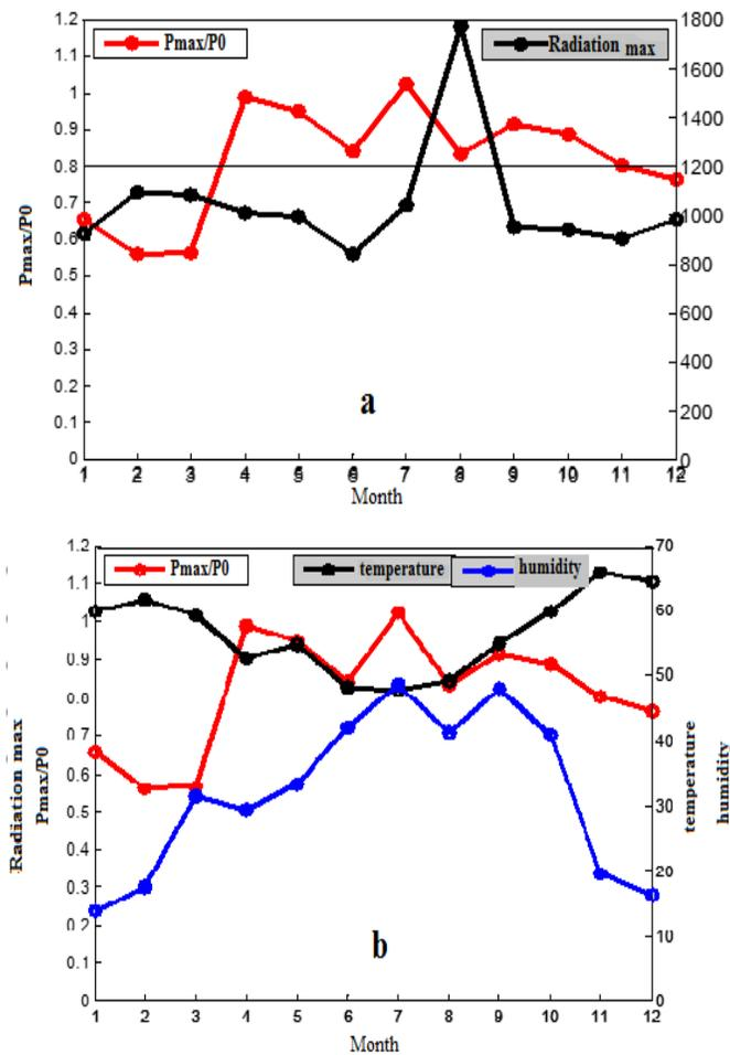
Fig. 12: Change in sunshine and degradation (a) Change in moisture and temperature and degradation (b)
