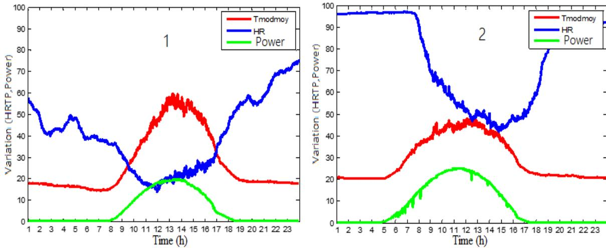
Fig. 6: Daily variation of temperature, relative humidity and power during a typical day during the dry season (1) and the rainy season (2)
