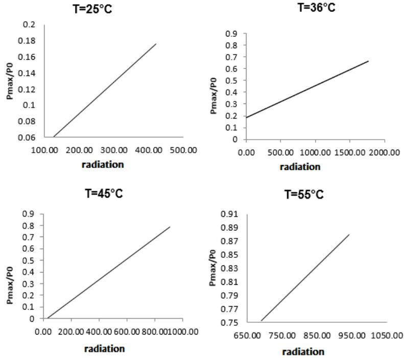
Fig. 13: Influence of radiation on the degradation at constant temperature
