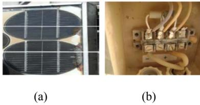
Fig. 3: PV module affected by corrosion of the edge (a) and the junction box (b)
