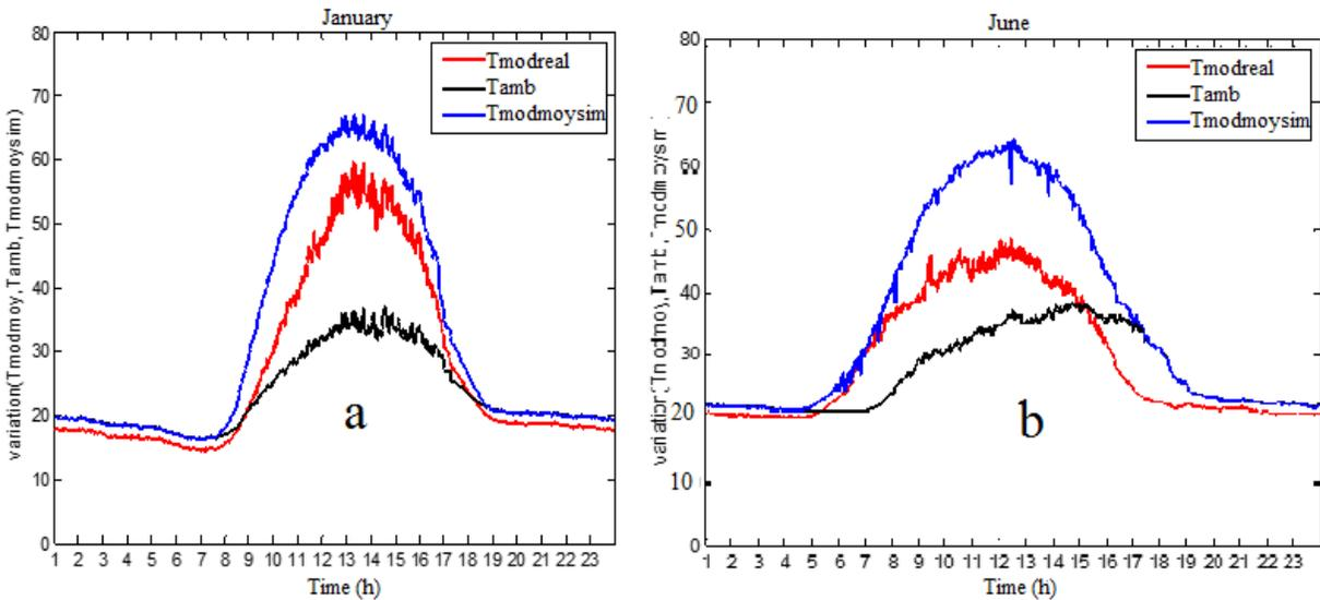
Fig. 9: Daily temperature variation of real and simulated modules and ambient temperature during the dry season (January-a) left and the rainy season (June-b) to right
