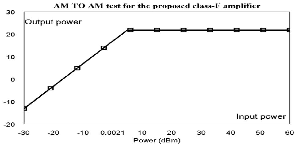
Fig. 7: Input and output power test (AM-AM test) for the proposed amplifier
