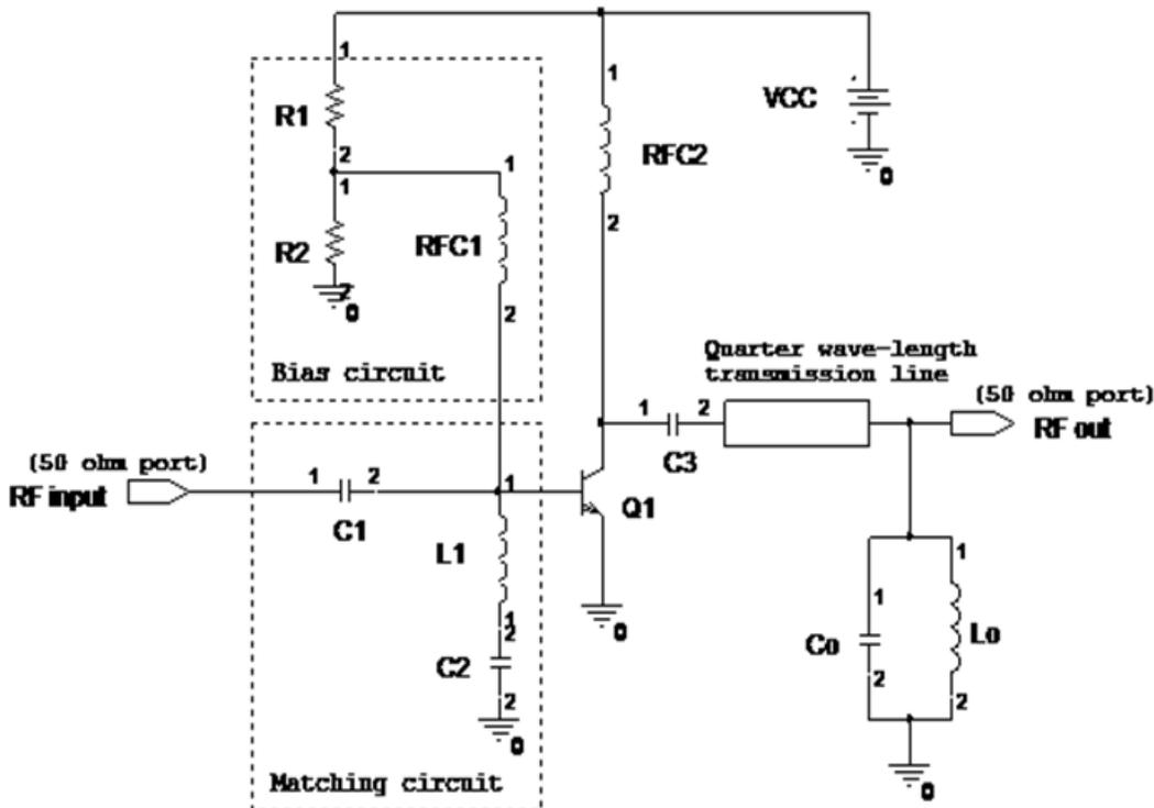
Fig. 1: The schematic design of the proposed class-F RF power amplifier
