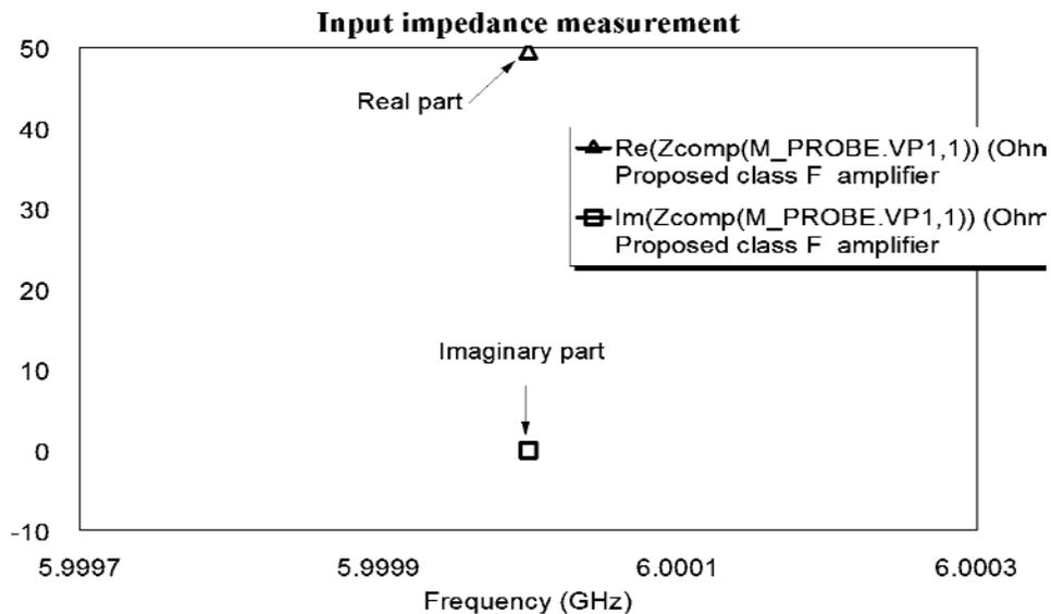
Fig. 3: The input impedance of the proposed amplifier with matching circuit
