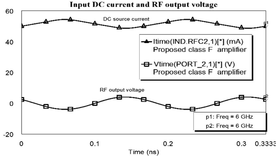
Fig. 8: DC source current and RF output voltage for an RF input of 5dBm
