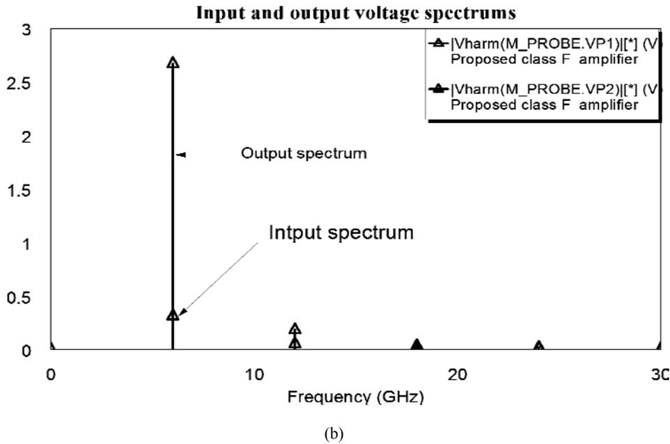
Fig. 5: Input and output voltages for an RF input of 0dBm; (a): actual waveforms and; (b): their spectrums
