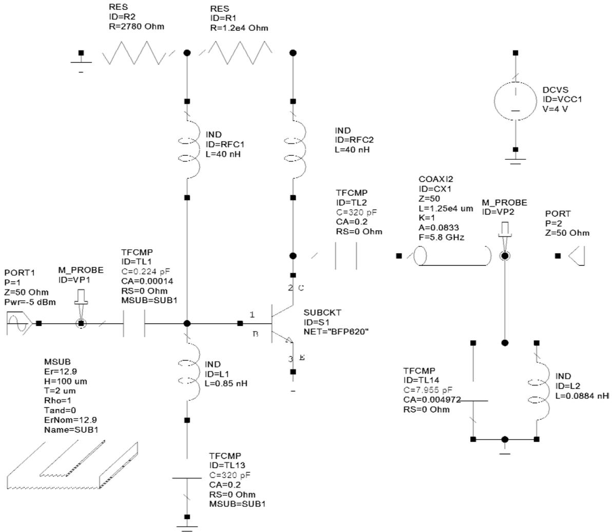
Fig. 2: The proposed amplifier circuit design using microwave office environments
