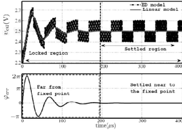
Fig. 4: Comparison of the ED and linear model of VSCP-PLL
