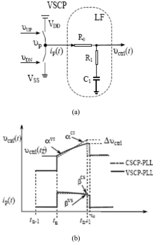
Fig. 3: (a): The VSCP-LF configuration; (b): The non-linear phenomenon of the VSCP comparing with the CSCP
