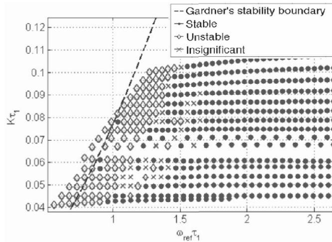
Fig. 7: The stability simulation results when  $v_{crit} > V_{DD}/2$  with symmetrical current  $I_p = i_p^{up}$
