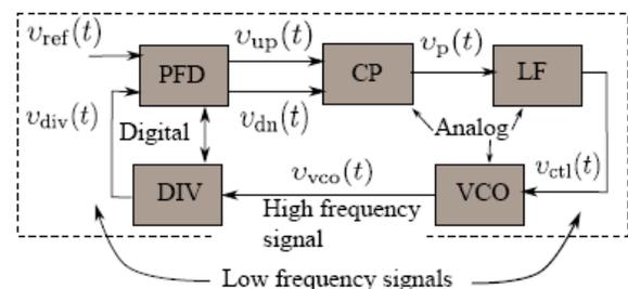
Fig. 1: The basic blocks of the CP-PLL for frequency synthesis
