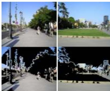
Fig. 3: Effect of RGB static filter on dataset DS. First row: Original images, Second row: result of applying the RGB static filter. The black pixels show the pixels reported as the non-sky pixels by the algorithm
