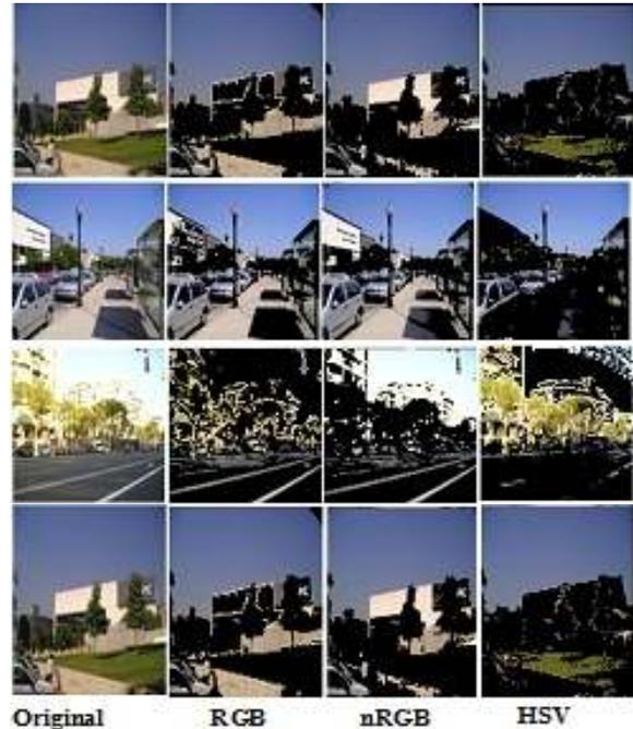
Fig. 10: Visualization effect of all the three static filters. First column: Original images, Second Column: RGB static filter, Third Column: nRGB static Filter, Fourth Column: HSV static filter
