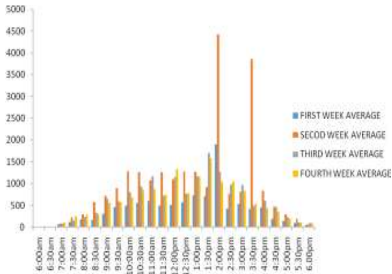
Fig. 5: Bar graph of the weekly average of solar radiation ( W/m^2 ) versus time (Min.) for September, 2015 at Prescocampus of Ebonyi State University, Abakaliki
