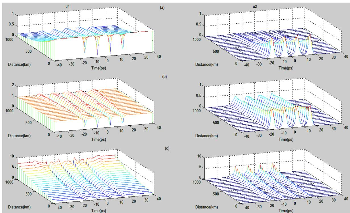
Fig. 4: The normalized four vector soliton intensity versus the propagation distance, (a)  $\gamma = -0.2$  and  $\alpha = 0$ , (b)  $\gamma = 0$  and  $\alpha = 0$ , (c)  $\gamma = 0.2$  and  $\alpha = 0$
