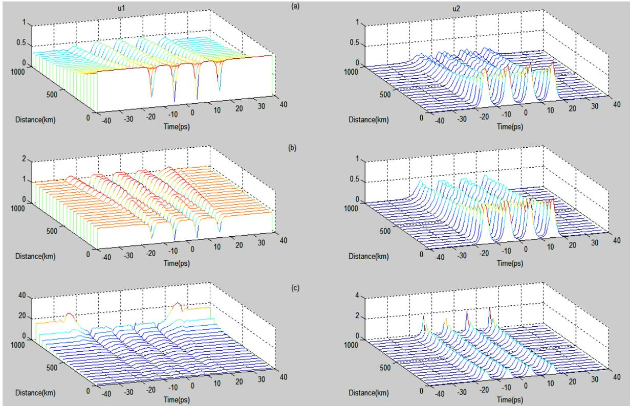
Fig. 5: The normalized four vector soliton intensity versus the propagation distance, (a)  $\gamma = 0$  and  $\alpha = -0.2$ , (b)  $\gamma = 0$  and  $\alpha = 0$ , (c)  $\gamma = 0$  and  $\alpha = 0.2$
