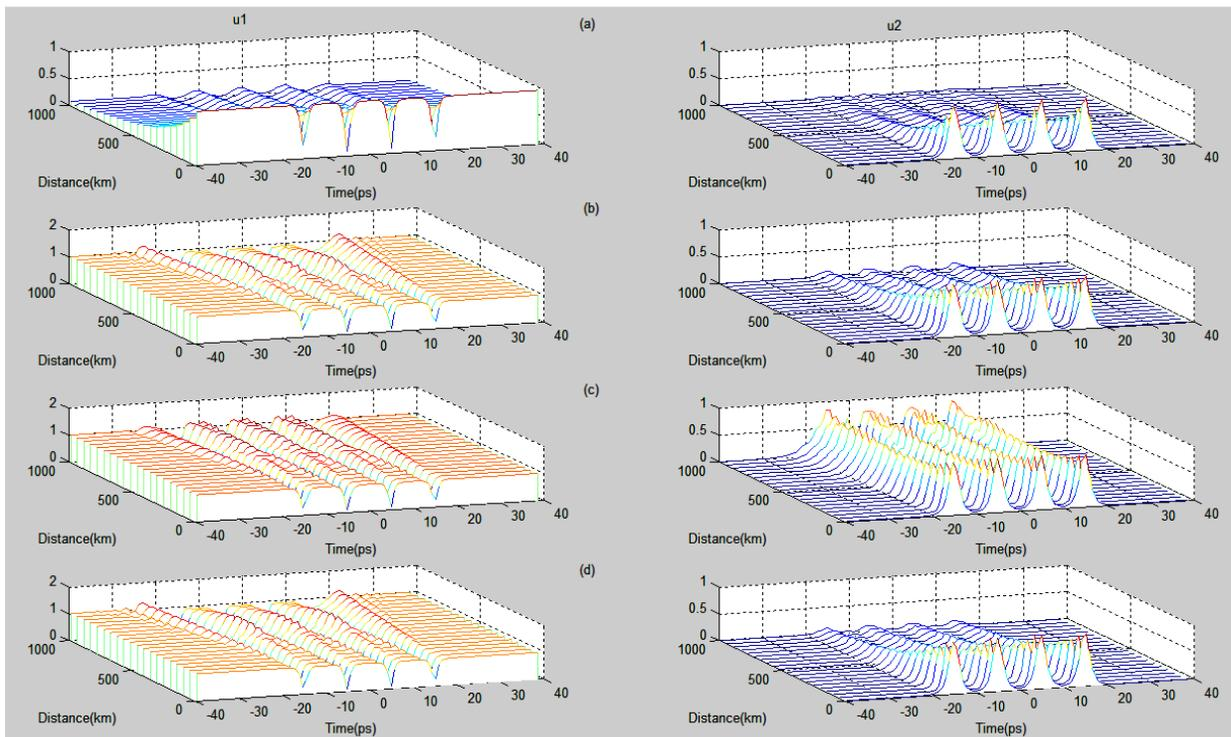
Fig. 6: The normalized four vector soliton intensity versus the propagation distance, (a)  $\gamma = -0.2$  and  $\alpha = -0.2$ , (b)  $\gamma = -0.2$  and  $\alpha = 0.2$ , (c)  $\gamma = 0.2$  and  $\alpha = -0.2$ , (d)  $\gamma = 0.2$  and  $\alpha = 0.2$
