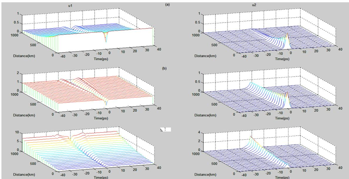
Fig. 1: The normalized vector soliton intensity versus the propagation distance, (a)  $\gamma = -0.2$  and  $\alpha = 0$ , (b)  $\gamma = 0$  and  $\alpha = 0$ , (c)  $\gamma = 0.2$  and  $\alpha = 0$
