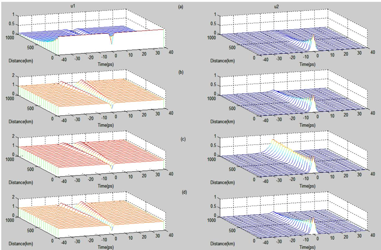
Fig. 3: The normalized four vector soliton intensity versus the propagation distance, (a)  $\gamma = -0.2$  and  $\alpha = -0.2$ , (b)  $\gamma = -0.2$  and  $\alpha = 0.2$ , (c)  $\gamma = 0.2$  and  $\alpha = -0.2$ , (d)  $\gamma = 0.2$  and  $\alpha = 0.2$
