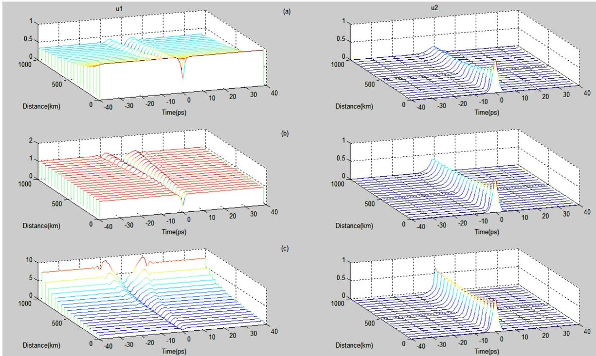
Fig. 2: The normalized vector soliton intensity versus the propagation distance, (a)  $\gamma = 0$  and  $\alpha = -0.2$ , (b)  $\gamma = 0$  and  $\alpha = 0$ , (c)  $\gamma = 0$  and  $\alpha = 0.2$
