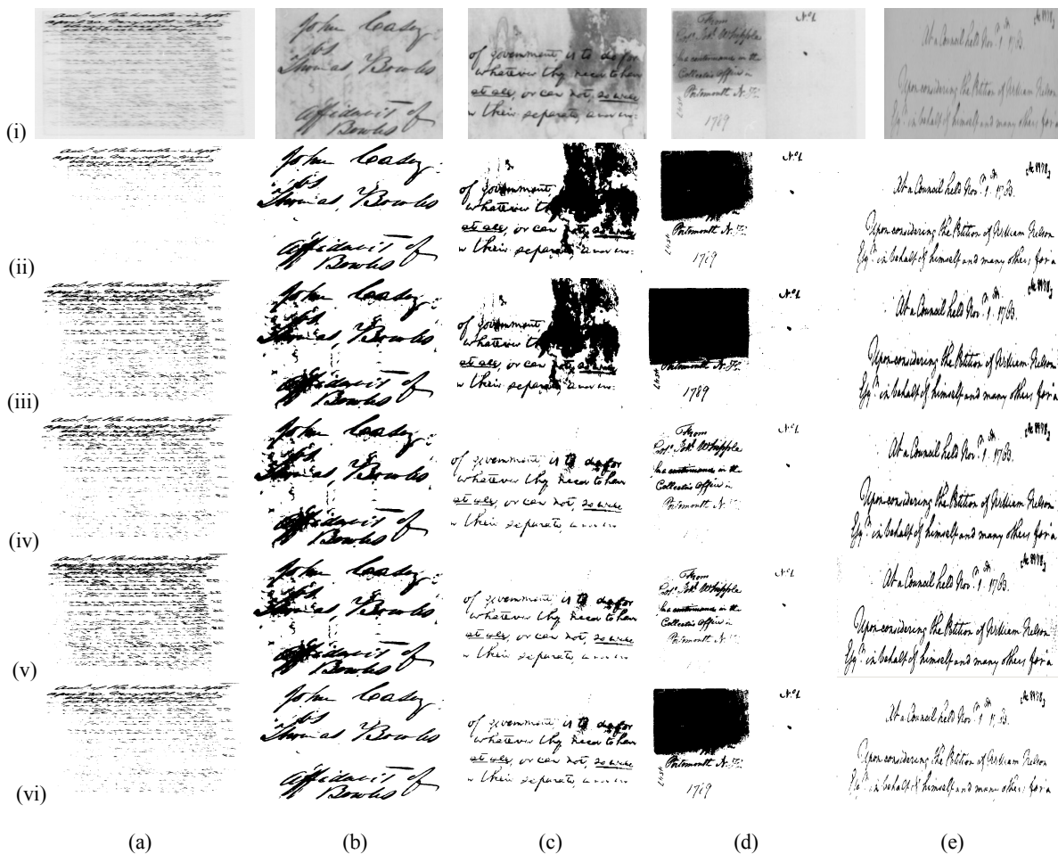
Fig. 3: (i) The DIBCO (2009) handwritten images: b, c and d are spotted and low-quality images; a, c and e are thin pen stroke, low-contrast and small-sized images. Also shown are the image results obtained using the (ii) Otsu (1979), (iii) Kittler and Illingworth (1986), (iv) Max entropy (Pun, 1980), (v) Potential difference (Acharya and Sreechakra, 1999) and (vi) proposed thresholding methods
