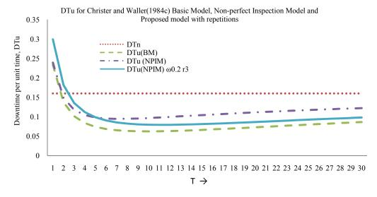
Fig. 5: Improvement of optimal DT<sub>u</sub> for soft repetitions with ω0.2, r = 3 in comparison to Basic delay time model, Non perfect inspection models; DTn (T∞, 0.16), DTuBM (T10, 0.06222), DTuNPIM (T7, 0.094598), DTuNPMIw0.2r3 (T11, 0.07911)
