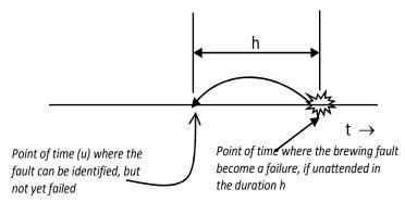
Fig. 1: Concept of delay time
