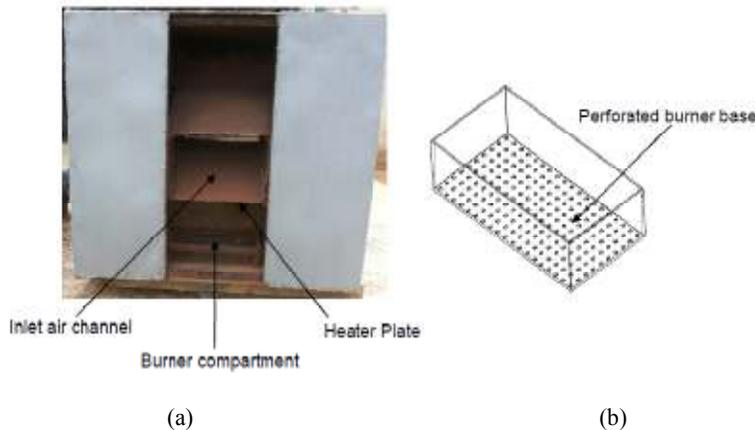
Fig. 2: The Kiln showing; (a): The heating section; (b): The burner
