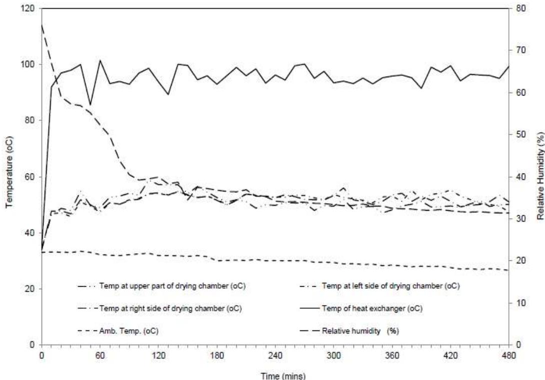
Fig. 4: The dryer performance when unloaded
