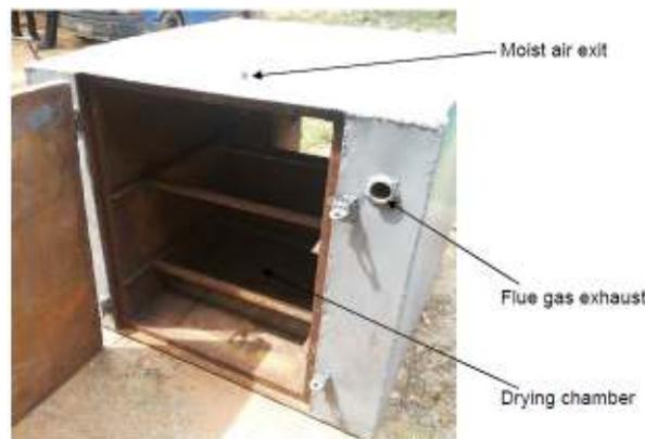
Fig. 3: The Kiln showing the drying section
