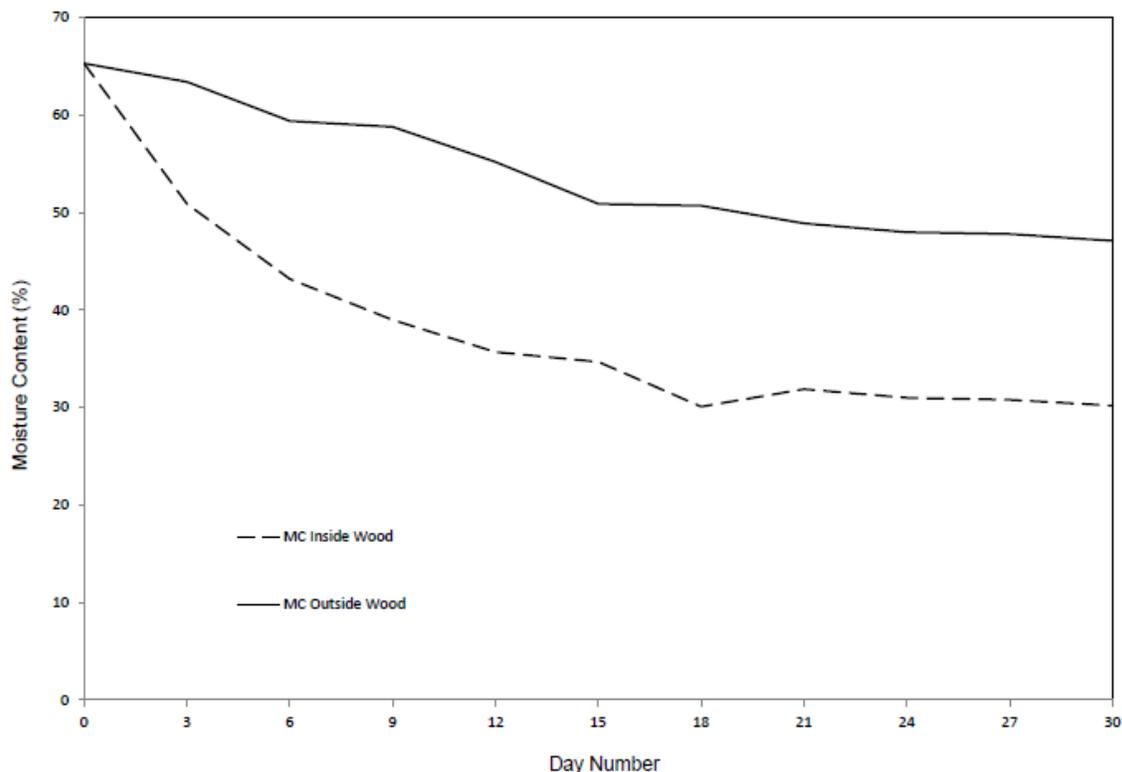
Fig. 7: Comparison of the wood moisture content variation during open air and kiln drying operations
