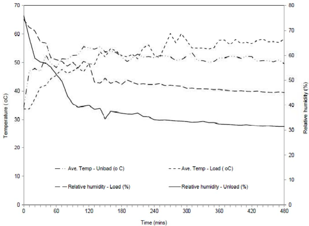
Fig. 6: Comparison of the loaded and unloaded dryer performance
