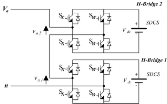
Fig. 1: A single phase multilevel inverter system
