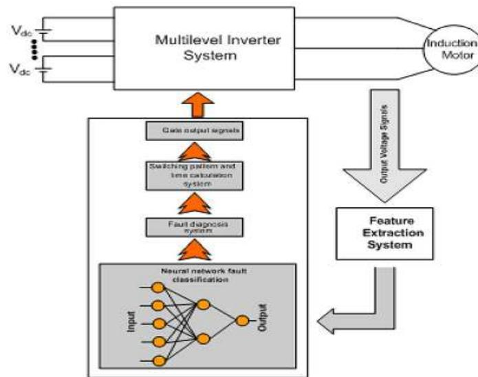
Fig. 3: Structure of fault diagnostic system
