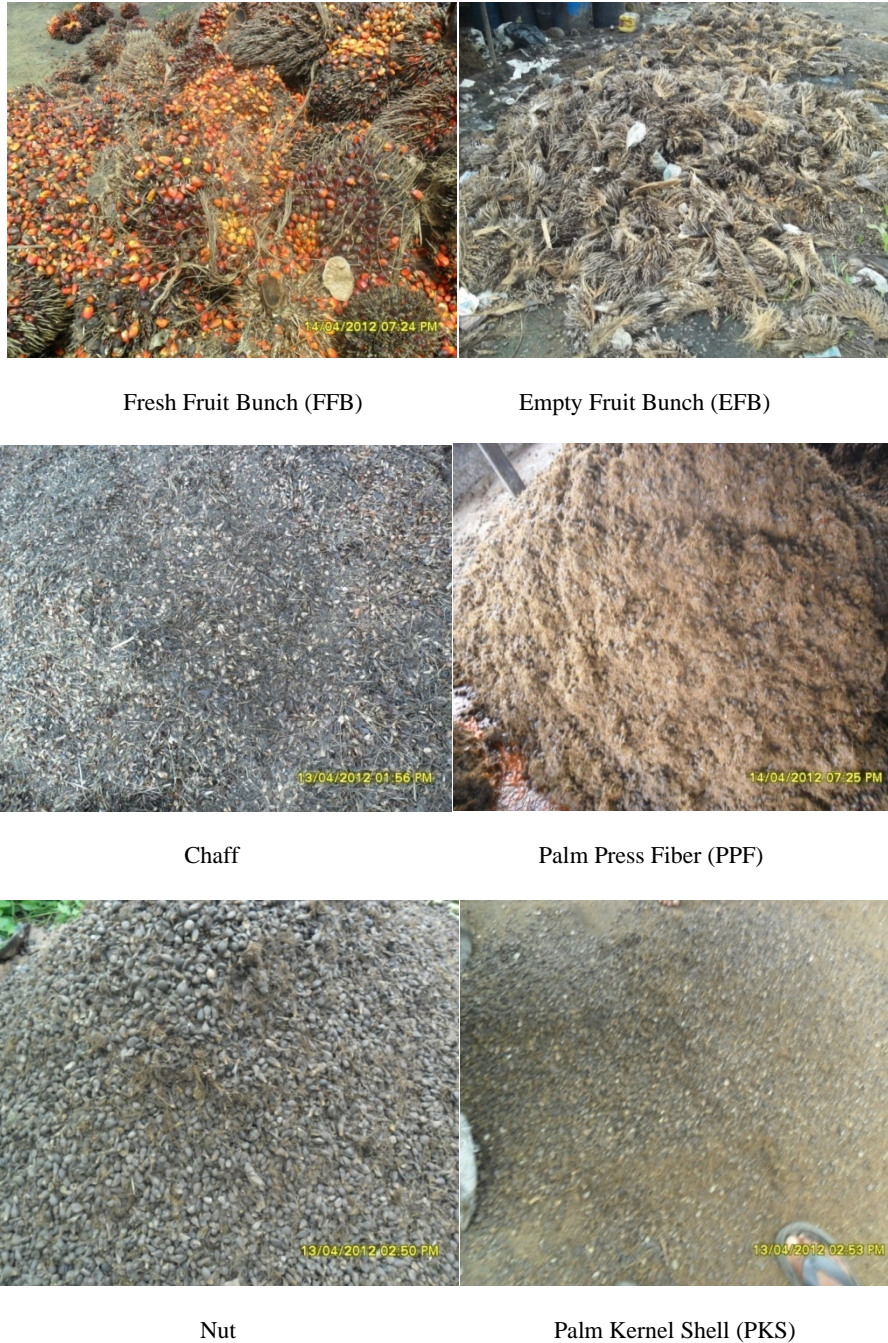
Fig. 2: Processing intermediates from FFB of oil palm
