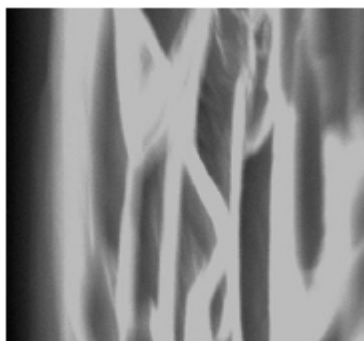
Fig. 4: Cross-sectional SEM image (1 x 1 μm 2 ) of porous silicon etched at 571 mA.cm -2 for 8 sec.
