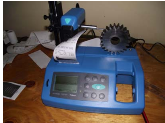
Fig. 15: Roughness testing measuring machine
