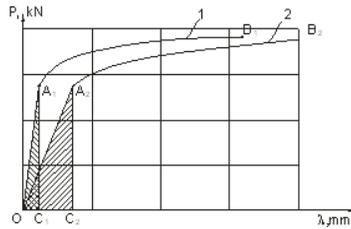
Fig. 1: Working characteristics of the elastic system: 1-System with no shock absorber, 2- System with shock absorber
