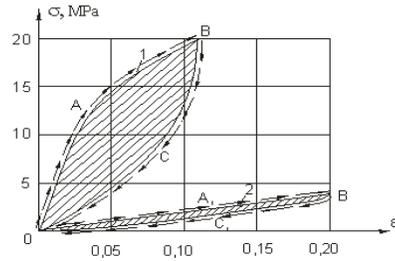
Fig. 3: Stress-strain diagrams of polyurethanes in compression
