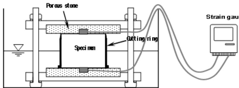
Fig. 3: Layout of the constant volume test apparatus
