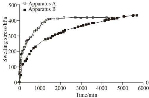
Fig. 6: Change processes of swelling stress with time
