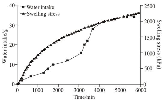
Fig. 4: Water intake and swelling stress evolution in the test
