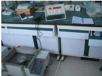
Fig. 2: Apparatus B: Constant volume test apparatus for swelling stress
