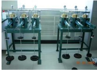
Fig. 1: Apparatus A: WG high-pressure triple combination consolidometer
