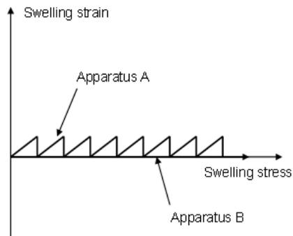
Fig. 5: Paths of the two methods for measuring swelling stress
