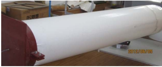
Fig. 6: Snapshot of inflatable fabric beam test setup
