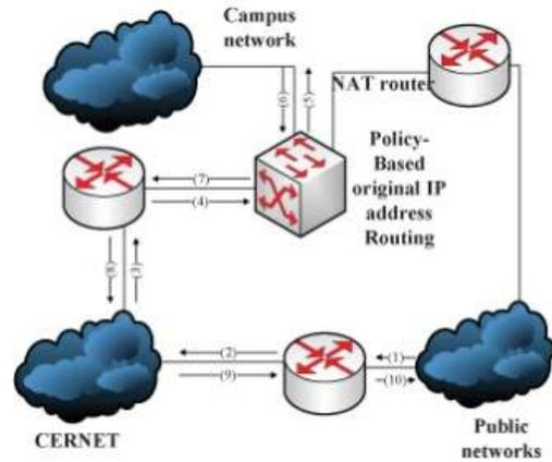
Fig. 3: A path to the campus network when access to a server with the PBR
