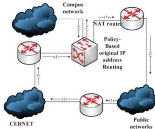
Fig. 4: A path to the campus network when access to a server without the PBR
