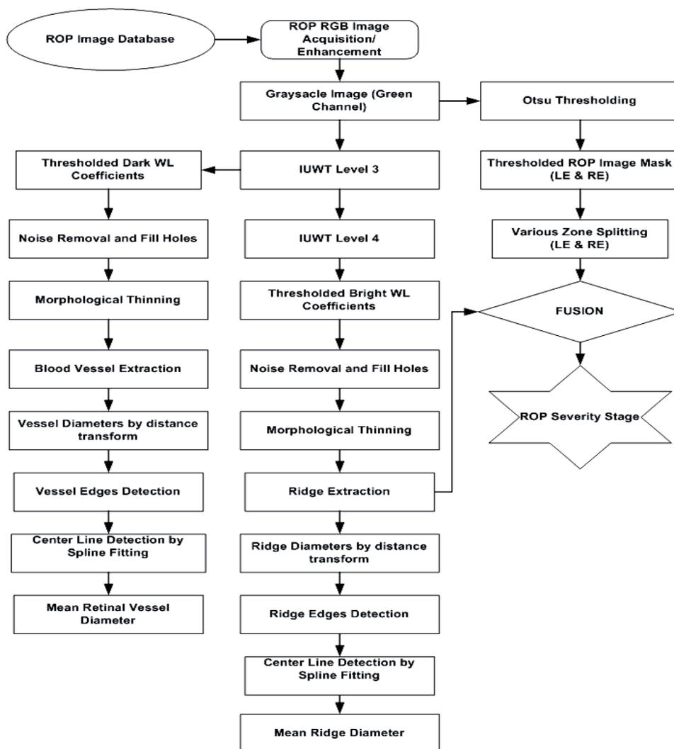
Fig. 3: General block diagram of wavelet based ROP screening system
