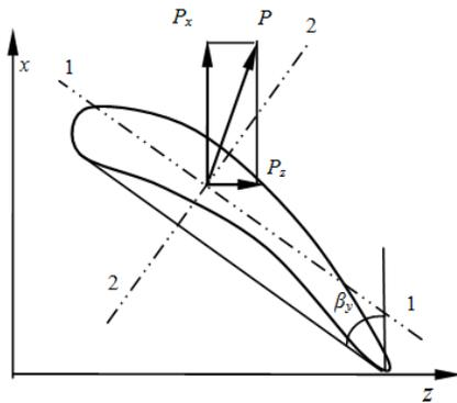
Fig. 5: Steam force on blade
