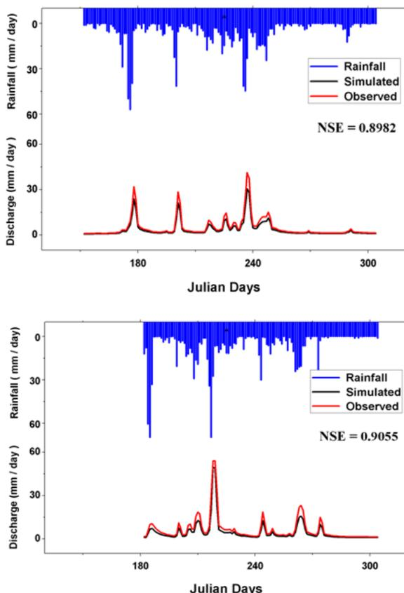
Fig. 4: Observed and simulated hydrographs of wardha watershed during calibration and validation period
