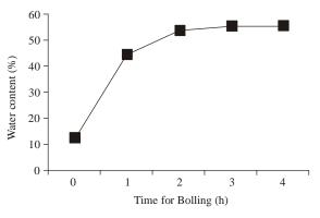
Fig. 3: Water content over coffee beans boiling
