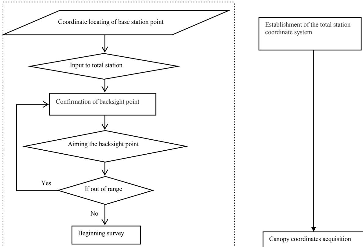
Fig. 2: Steps in determining the total station coordinates
