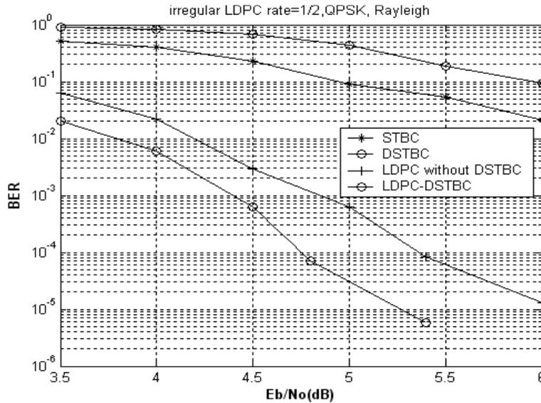
Fig. 3: Performance of the LDPC-DSTBC for QPSK modulation
