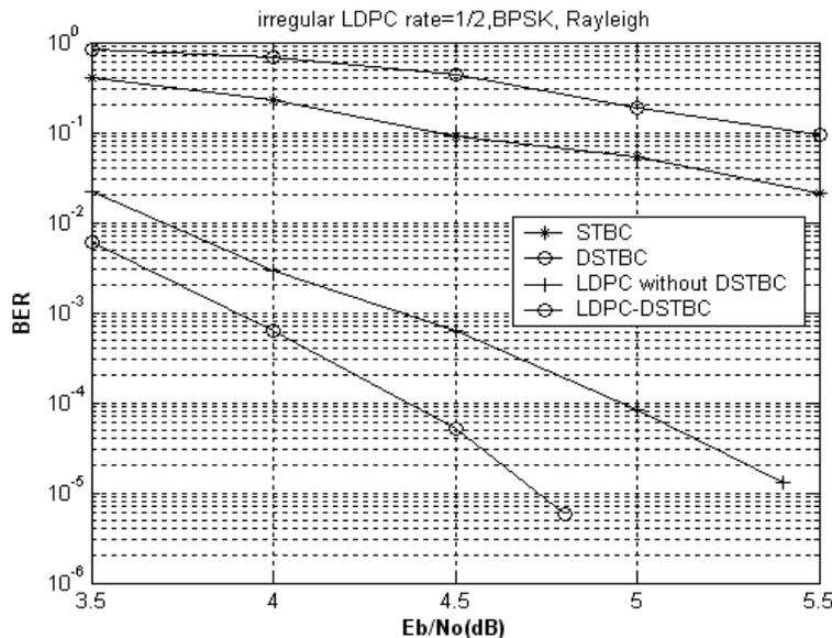
Fig. 2: Performance of the LDPC-DSTBC for BPSK modulation
