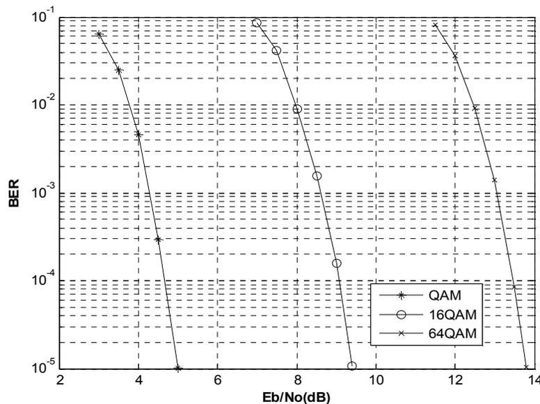
Fig. 4: Performance of the LDPC-DSTBC for code rate 1/2 (1008, 504)
