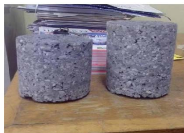
(b) Filed cores of PCC pavement
