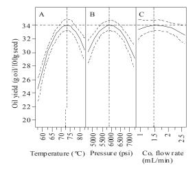
Fig. 3: Determination of the optimum values for temperature (A, 73°C), pressure (B, 5,900psi) and CO<sub>2</sub> flow rate (C, 1.5 mL/min).
