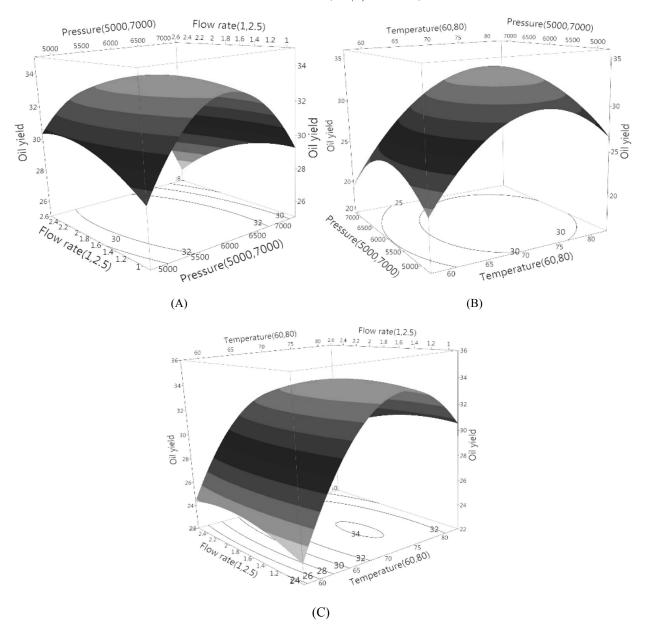
Fig. 2: Response surface curve and its contour plot for; (A): the effects of temperature and pressure at a constant CO<sub>2</sub> flow rate of 1.75 mL/min; (B): the effects of pressure and CO<sub>2</sub> flow rate at a constant temperature of 70°C; (C): the effects of temperature and CO<sub>2</sub> flow rate at a constant pressure of 6,000psi (41,369 kPa) on the oil yield
