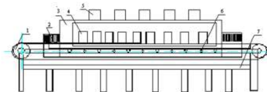
Fig.1: The whole structure figure of microwave sterilizer; 1-the conveyor belt, 2- the microwave leakage control mechanism, 3- the microwave sterilizer, 4-the observation window, 5- the microwave generator, 6-the splined shaft, 7- framework
