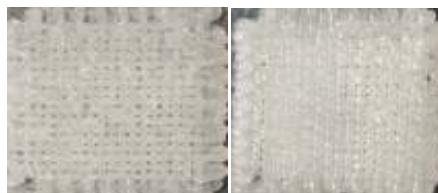
Fig. 3: Scaffold made of gelatin and sodium alginate
