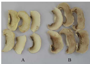
Fig. 4: Color quality of 0.08% glutathione (a) and control (b) samples
