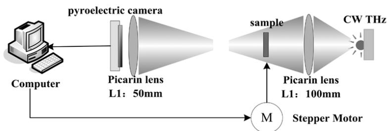
Fig. 1: Experimental installation figure
