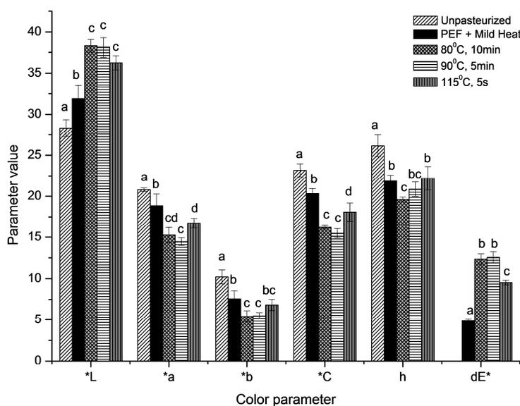
Fig. 3: Comparison between combined PEF with mild temperature (optimized conditions) and conventional pasteurization on red apple juice color parameters. Means with different letters were significantly different (p<0.05)
