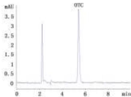
Fig. 1: Chromatograms of OTC standard (1µg/mL)
