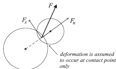
Fig. 2: Contact logic
