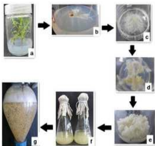
Fig. 5: Schematic diagram of suspension cells culture system initiated from hairy roots; (a) Aseptic seeding of P. tunicoides , (b) Hairy root induction, (c) Liquid culture of hairy roots, (d) Induction of hairy root-derived callus, (e) Hairy root-derived callus cultured on solid media, (f) Suspension cells cultured in a shaking-flask, (g) Suspension cells cultured in a 2.5 L micro-bubbling bioreactor
