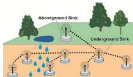
Fig. 1: Usage of wireless underground sensor networks for agricultural monitoring
