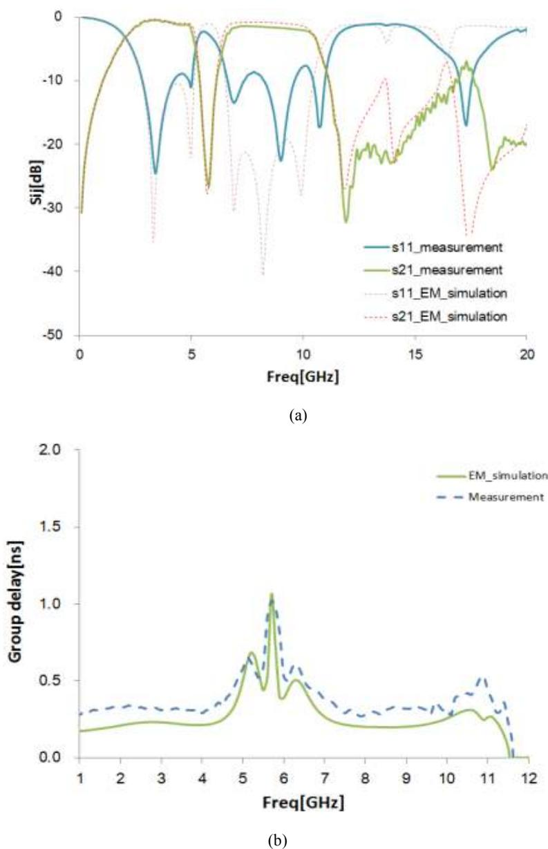
Fig. 6: Simulated and measured frequency responses of UWB BPF; (a): Wideband amplitude response; (b): Group delay
