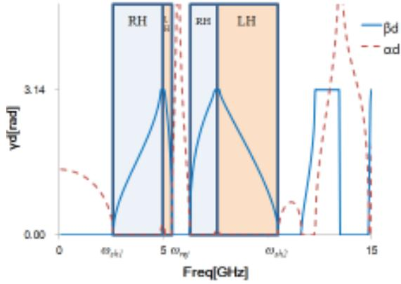
Fig. 3: Dispersion and attenuation diagram of distributed CRLH TL unit cell
