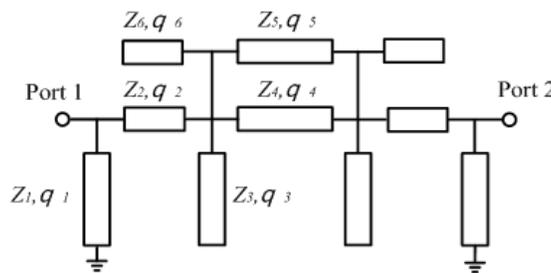
Fig. 1: Distributed CRLH TL unit cell for notched UWB BPF
