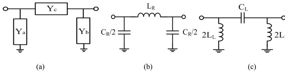
Fig. 2: (a):  $\pi$  equivalent circuit of distributed CRLH TL unit cell; (b): Equivalent circuit when  $Y_a, Y_b > 0$  and  $Y_c < 0$ ; (c): Equivalent circuit when  $Y_a, Y_b < 0$ , and  $Y_c > 0$
