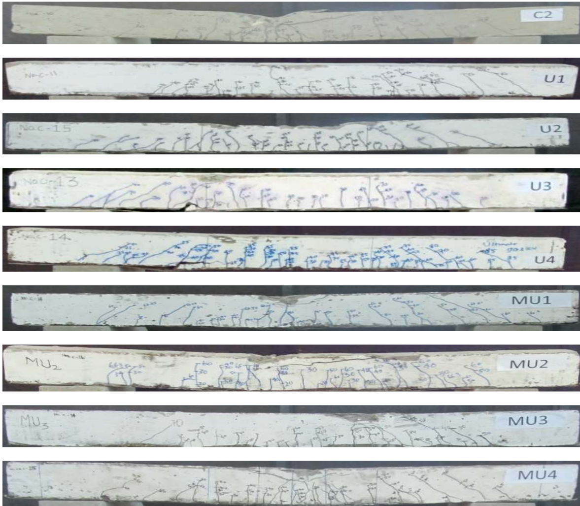
Fig. 23: Failure crack pattern of reference and strengthened beams
