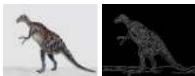
Fig. 3: Edge map for the dinosaur category of the corel dataset using canny edge detection, the parameters used are standard deviation ( \sigma = 1.4 , low threshold = 0.5, high threshold = 2.5, sigma = 1)
