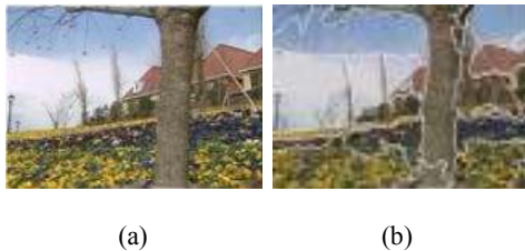
Fig. 5: JSEG segmentation methods; (a) The original image, (b) Image segment with 27 regions (Serra, 2003)
