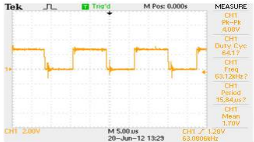
Fig. 7: PWM pulse from TL494 during switching
