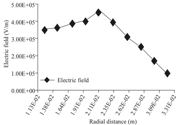
Fig. 9: The plot of electric field vs radial distance for the cable with air void
