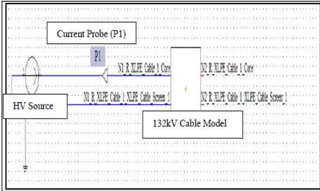
Fig. 10: Circuit diagram for simulation using CST cable
