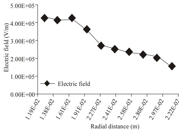
Fig. 7: The plot of electric field vs. radial distance for the cable with no air void
