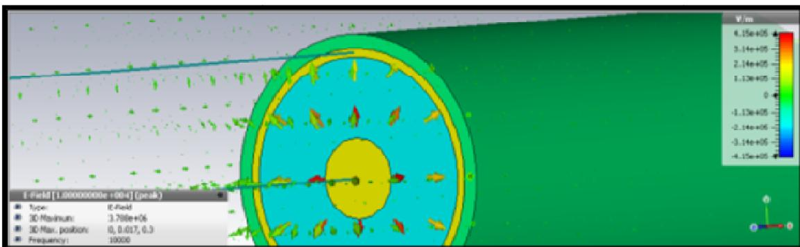
(a): Electric Field 3D Vector Plot without air voids
