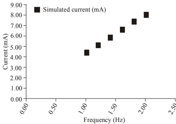
Fig. 11c: Current vs. frequency results for 6kV from 1 to 2 kHz
