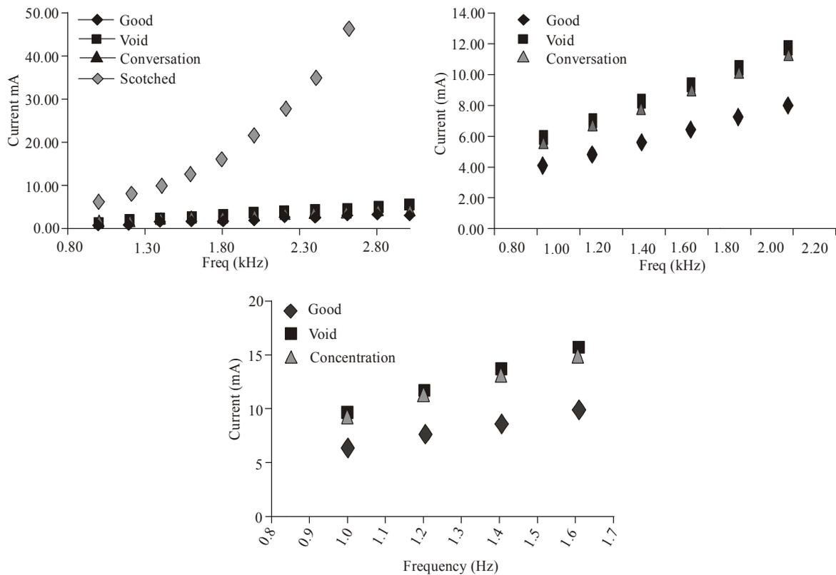
Fig. 17: Current vs. Frequency for; (a): 2kV; (b): 6kV; (c): 10 kV
