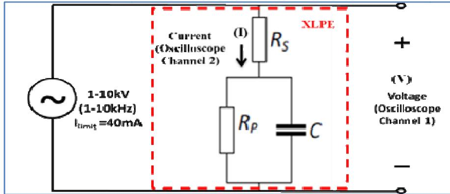
Fig. 2: Equivalent circuit of tan delta measurement method of a cable
