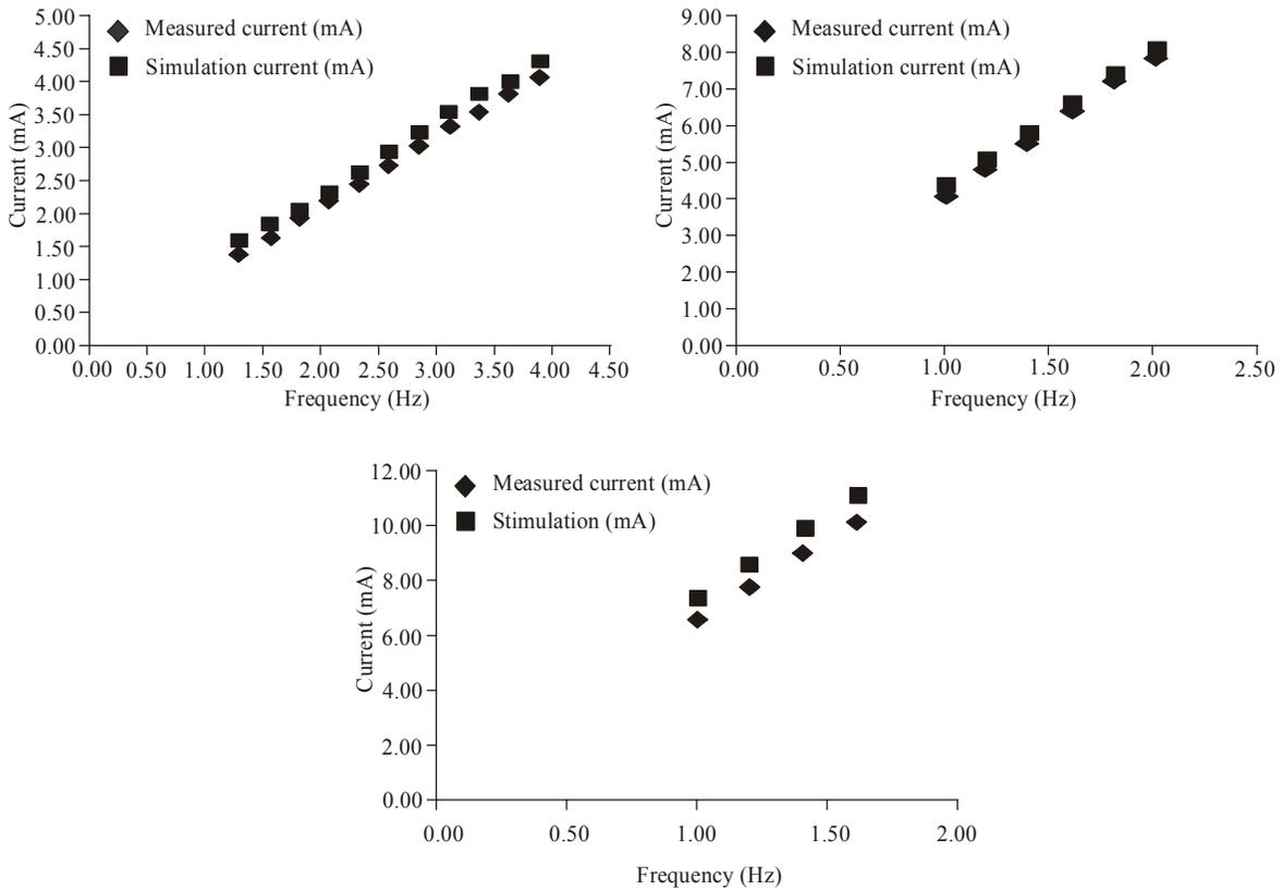
Fig. 18: Current vs. Frequency simulated and measured for; (a): 2kV; (b): 6kV; (c): 10kV good cables
