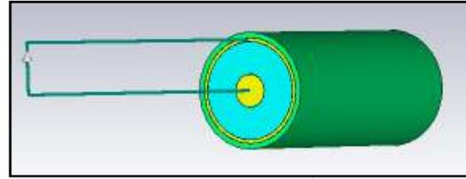
Fig. 5: The cable model for the electric field simulation
