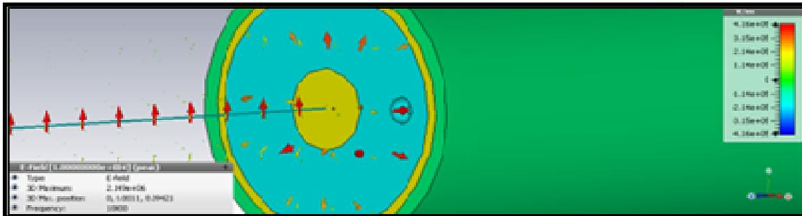
(a): Electric Field 3D Vector Plot with air void
