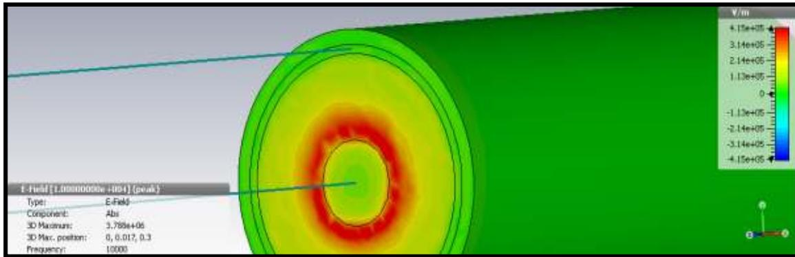
(b): Electric Field 3D Scalar Plot without air voids
