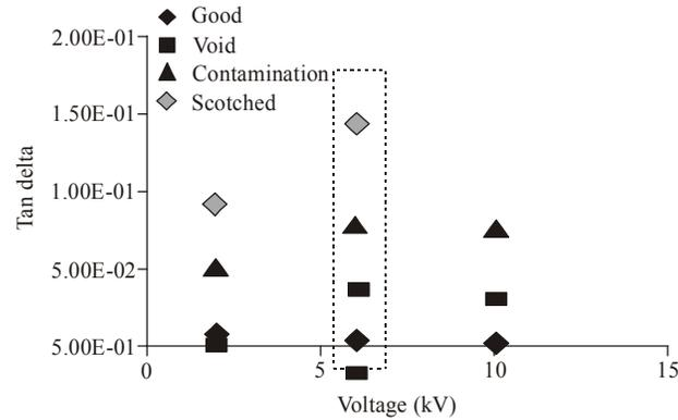
Fig. 20: Tan delta vs voltage at 1kHz
