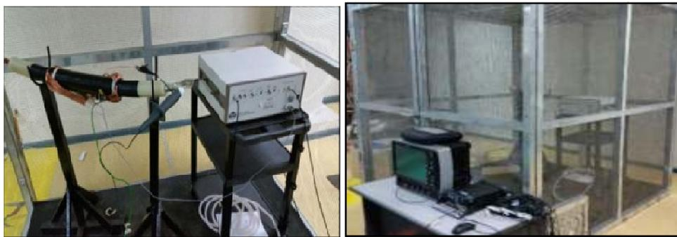
Fig. 15: Laboratory setup for HF tan delta measurement system
