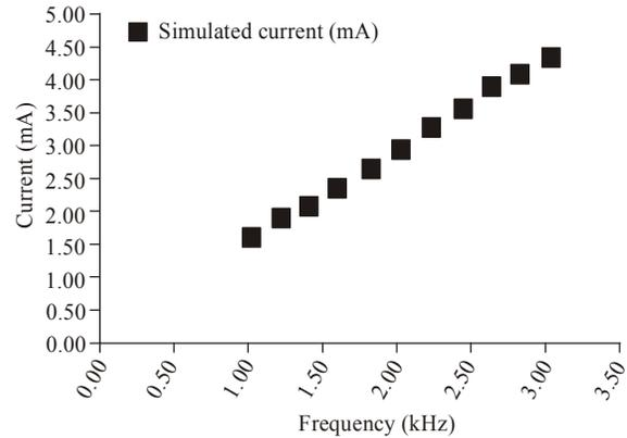
Fig. 11b: Current vs. frequency results for 2kV from 1 to 3 kHz
