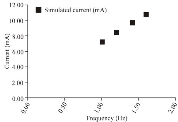
Fig. 11d: Current vs. frequency results for 10kV from 1 to 1.6 kHz
