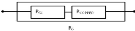
Fig. 3: Equivalent modal of  $R_S$
