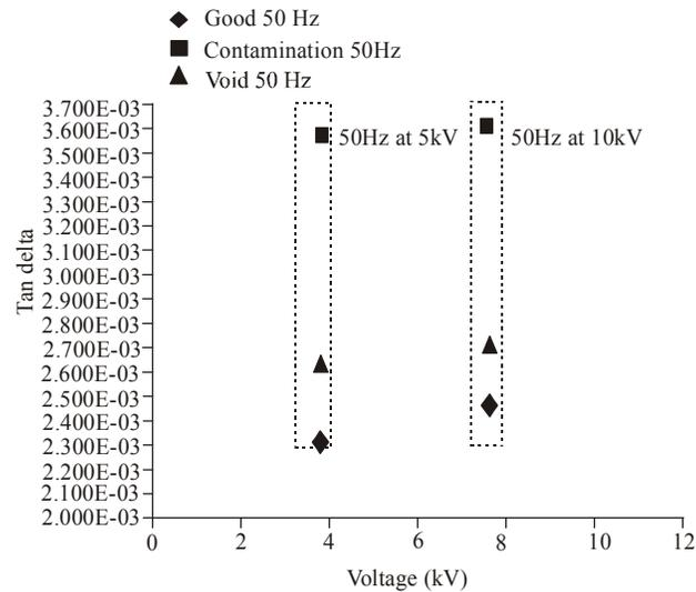
Fig. 21: Tan delta vs. voltage at 50 Hz
