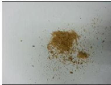
Fig. 13: Wood dust particle inserted into machine to create contaminated cable
